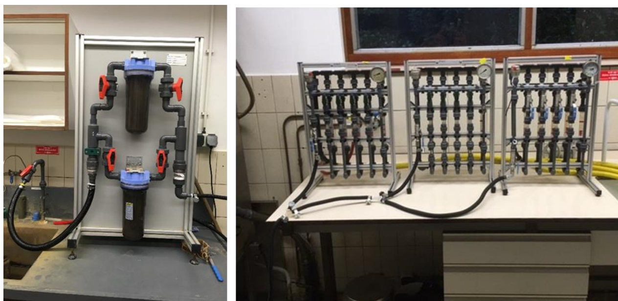
Figure 3-1. Installation of three CBMs on surface water at Keizersveer. Left: the surface water is first filtrated over a candle filter. Right: Three CBMs (of KWR) that receive the filtrate of the candle filter.
