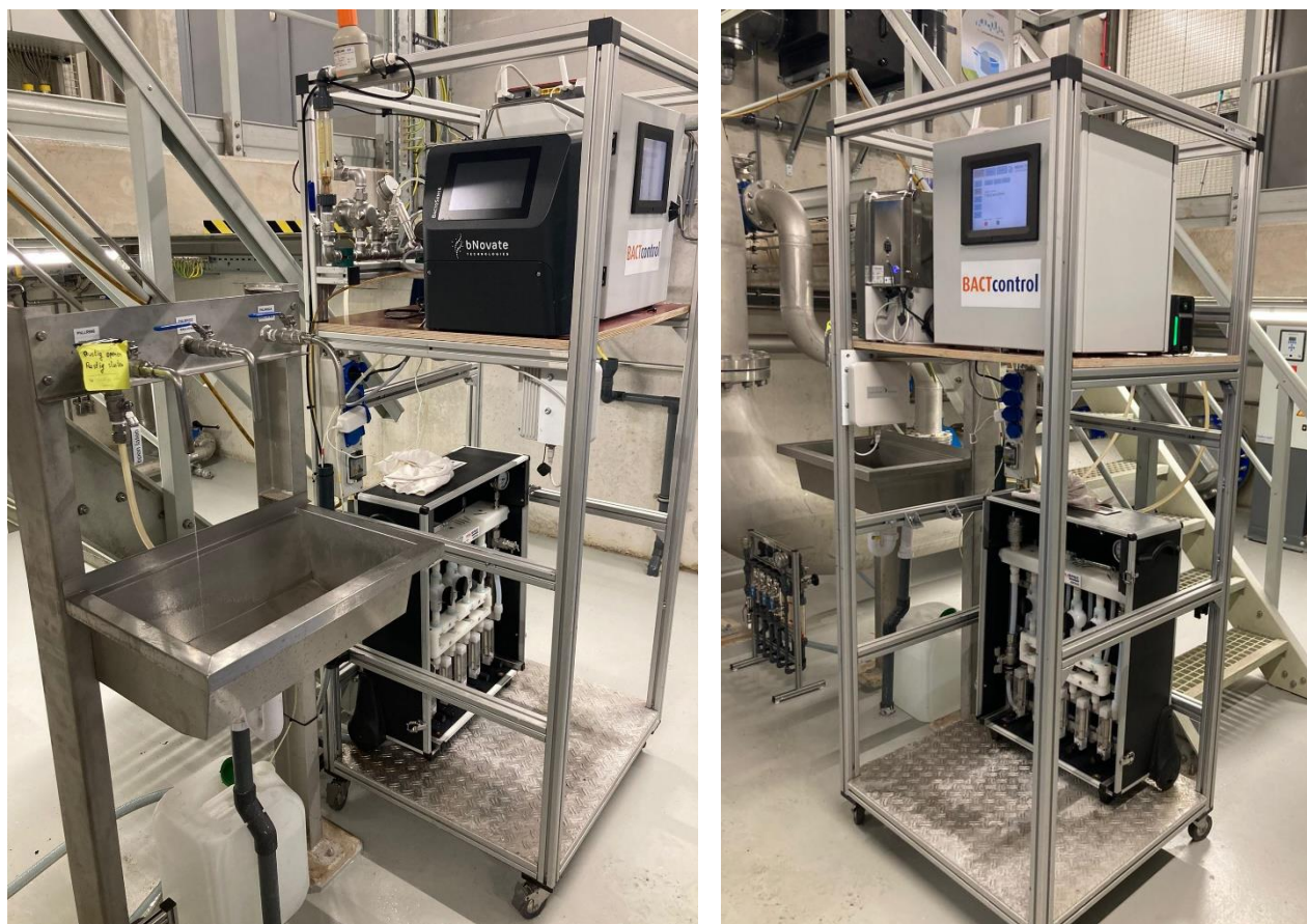
Figure 5-3. Installation of BACTcontrol, BactoSense, KWR-CBM and Milispec-CBM at production location Nieuw-Lekkerland, Oasen.
