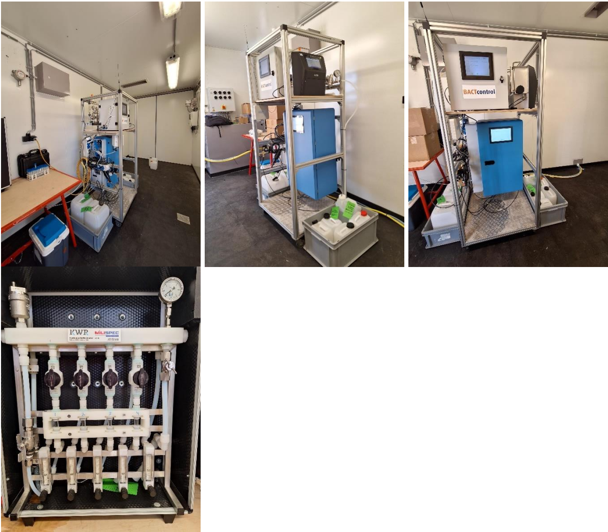
Figure 8-5: The sensors and the set-up in the container. Upper figures show the BactoSense, BACTcontrol and the BugCount Guardian. The lower picture shows the CBM.
